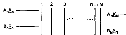
FIG. 2. Schematic of entering and exiting waves as a result of internal transmission and reflection processes within a series of density intervals.
