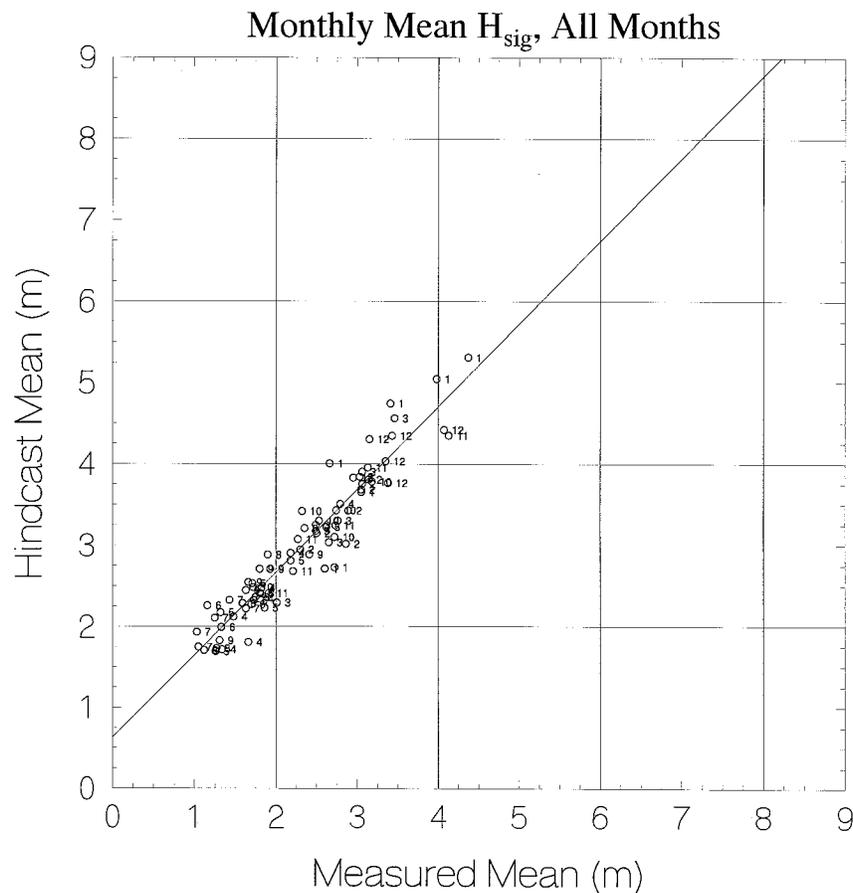
FIG. 1. Scatterplot of monthly averaged hindcast significant wave height at a grid point closest to SSLV vs observations there. Units are in m.
