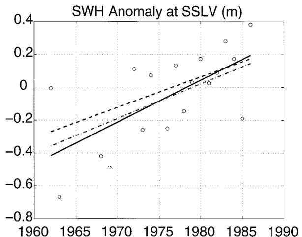
FIG. 5. The least squares linear trend fitted to cold-season (November–March) average SSLV observations (solid line) and the trend according to the statistical–dynamical hindcast at the closest grid point (dashed line). The dotted–dashed line is the trend fitted to hindcast data taken only for seasons with available SSLV observations. Also shown are the observed cold-season-averaged significant wave height anomalies at SSLV (circles). Abscissa is SWH anomaly in m.
