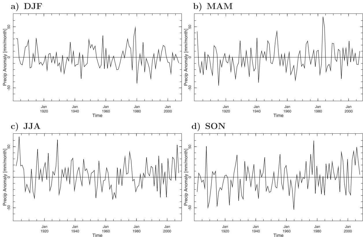
FIG. 2. The seasonal mean (DJF, MAM, JJA, and SON) precipitation anomalies relative to the long-term seasonal means for the Catskill Mountains and surrounding areas from the GPCC gridded data. Units are  $\text{mm month}^{-1}$ .
