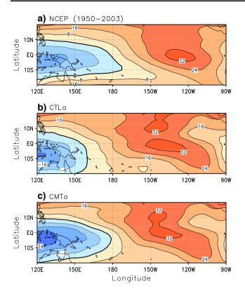
Fig. 3 DJF mean vertical wind shear over the tropical Pacific. Units are m/s. a NCEP, b CTLa and c CMTa
