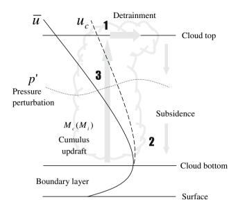
Fig. 1 Schematic diagram of an idealized convective grid cell with vertical wind shear. *Solid and dashed lines* represent environmental and in-cloud vertical wind structure, respectively. The convective scale pressure perturbation is also drawn (*dotted line*). *Arrows* represent mass fluxes. *Numbers* indicate the region where each term of Eq. (1) is active. See text for details
